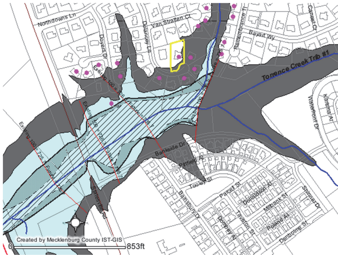
Figure AF-9 Charlotte-Mecklenburg, North Carolina, flood hazard map showing 1% annual chance flood hazard area (blue shaded area) and community flood hazard area based on future development upstream (gray shaded area). (Photo source: City of Charlotte)
