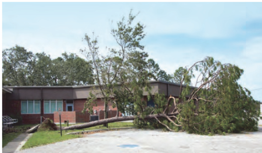
Figure H-16 Had this tree fallen in the opposite direction during 2004 Hurricane Ivan in Florida, it would have damaged the school (FEMA, 2007).
