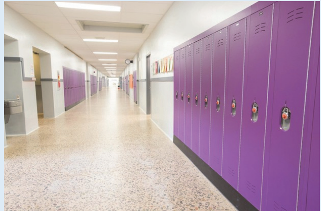
Figure F-7 Metal lockers were replaced with high density polyethylene (HDPE) lockers (Scranton Products, 2016).
