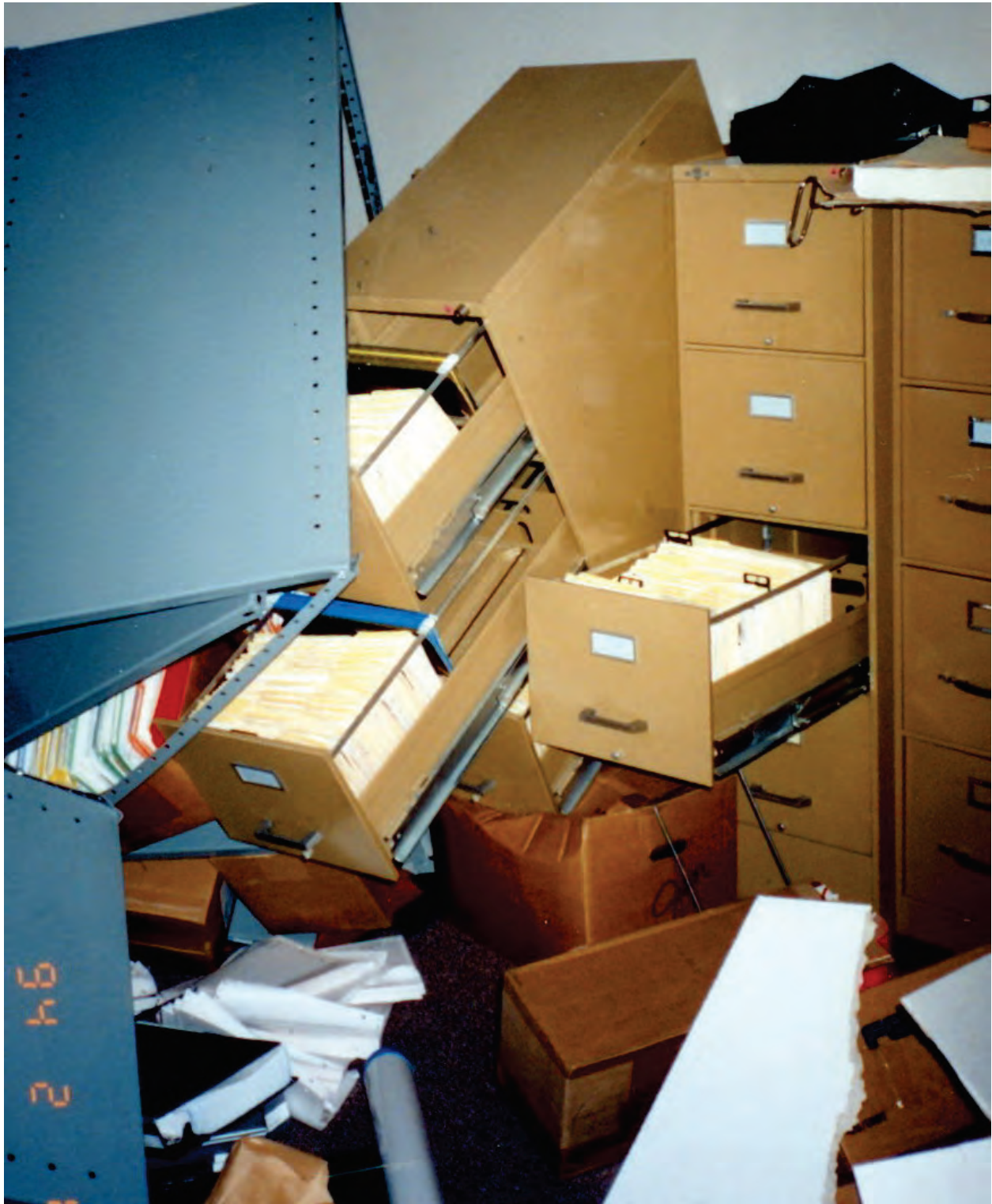
Figure 6.5.5.1-1 Failure of file cabinets in the 1994 magnitude-6.7 Northridge Earthquake (Photo courtesy of Wiss, Janney, Elstner Associates).
