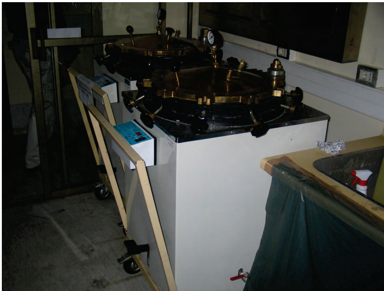
Figure 6.5.5.3-3 Equipment on wheels did well during the 2010 magnitude-8.8 Chile Earthquake; there were no reported injuries or examples of overturning related to equipment mounted on wheels. Centrifuges on wheels shown in photo (Photo and information courtesy of Bill Holmes, Rutherford & Chekene).
