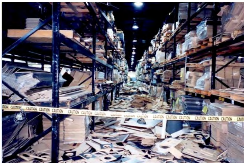
Figure 2.4.2-2 Damage to inventory on industrial storage racks in the 1994 Northridge Earthquake (FEMA 74, 1994).
