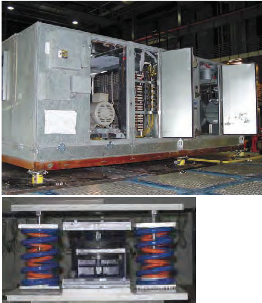
Figure 6.4.1.3-7 Seismic shake table testing of an air-handler unit and vibration isolation restraint system as part of the MCEER-ASHRAE project (Photos courtesy of André Filiatrault, MCEER).
