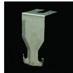
Figure 6.3.4.3-2a Complete collapse of a large suspended gypsum board ceiling over a swimming facility in Japan (Photo courtesy of Shojiro Motoyui, Tokyo Institute of Technology). This type of failure has been replicated on the E-defense shake table and occurs when the U-shaped clip holding the cross furring (M-bar) to the main runners (channel) opens into a V-shape and drops the furring grid. This type of failure is not common in the U.S.
