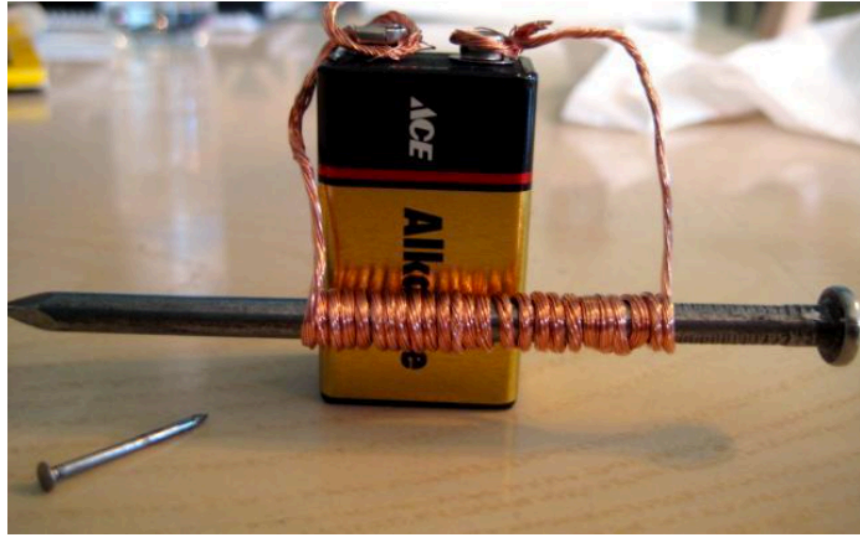
Electromagnet by Gina Clifford, CC BY-SA
